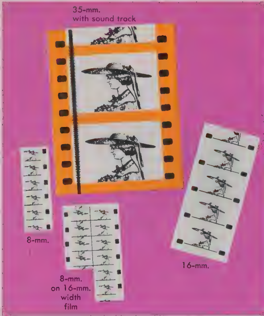
The most common motion-picture film sizes are those above, plus 70-mm., used for wide-screen projection. In production of a sound track (below), a microphone converts sound into electrical impulses. In magnetic recording, the impulses influence a magnetic field, the variations of which appear as a pattern on magnetized film. In optical recording, the impulses control the amount of light reaching sensitized film.
